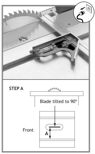
**Figure 93.** Making the first slot-to-blade measurement at 90°.
